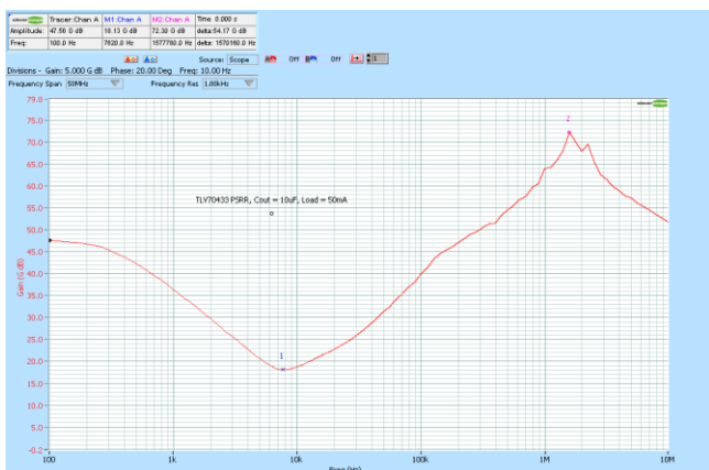
TLV70433 PSRR using CS1070 (1A 50 MHz op-amp):
